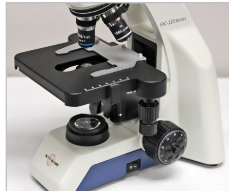
The stage size is 150mm x 139mm with a movement range of 75mm x 32mm
